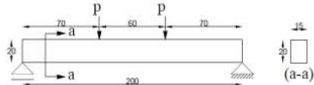
Figure 1. Rectangulaer concrete beam diagram
