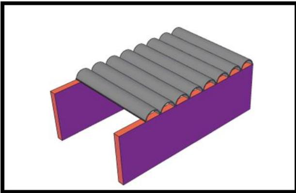
Fig .6 Finished Ferrocement Roofing Channel
