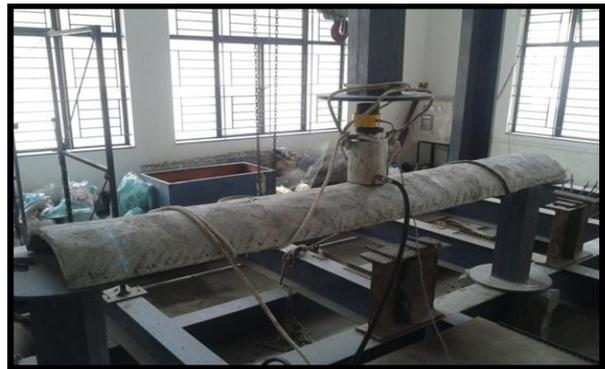
Fig. 7 Testing of ferrocement channel
