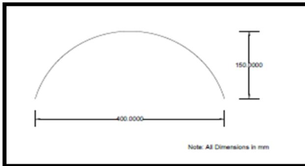
Fig. 1 Section of Ferrocement Channel
