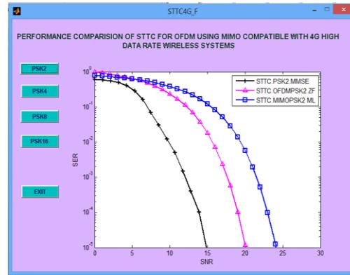
Figure 1 The relation of symbol error rate (SER) and SNR gain with 2- state PSK and conditions taken for decoding are MMSE and ZF and reduction of noise in transmission state.
