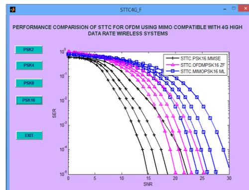
Figure 3 the relation of symbol error (SER) rate and SNR gain with 16- state PSK and conditions taken for decoding are MMSE and ZF and reduction of noise in transmission state.
