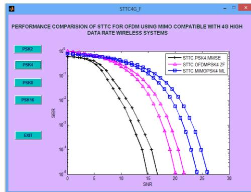
Figure 2 the relation of symbol error rate (SER) and SNR gain with 4- state PSK and conditions taken for decoding are MMSE and ZF and reduction of noise in transmission state.
