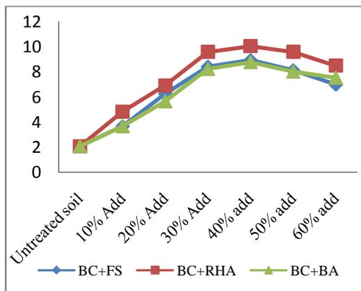
**Fig. 8 effect of wastes on CBR of soil**
