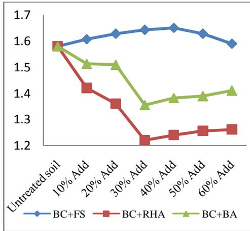
**Fig. 7 effect of wastes on MDD of soil**
