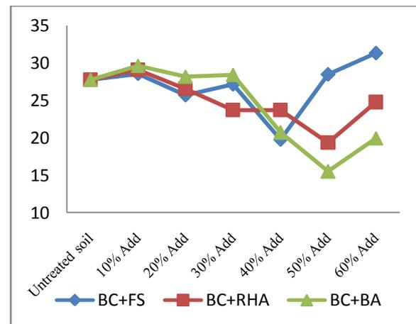
Fig. 6 effect of wastes on plasticity index of soil
