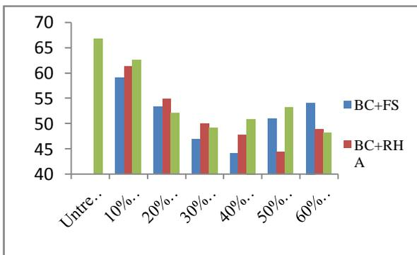
Fig. 5 effect of wastes on liquid limit of soil
