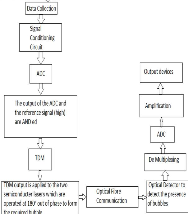
Fig. 1.0: Flow diagram indicating the process of Advanced Version of Li-Fi using LASERS
