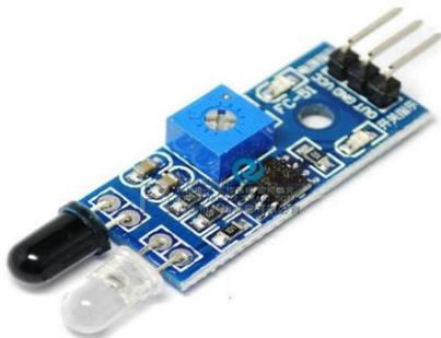
Figure 2: IR Sensor HDLC-4260
