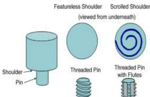
Fig.1. Schematic drawing of the FSSW tool.
