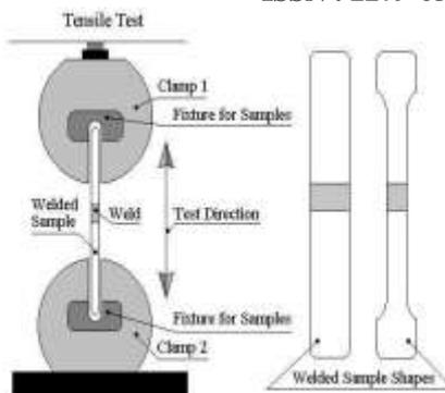
Fig. 4. (a) Tensile Machine, (b) Schematic diagram of tensile specimen and Fixture.
