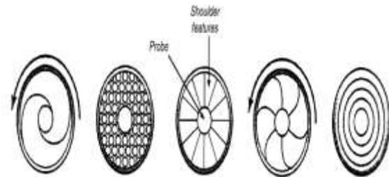
Fig .2. Tool shoulder geometries, viewed from underneath the shoulder.
