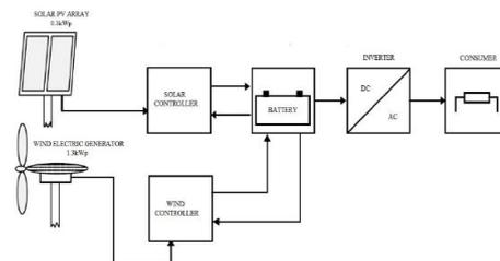
Figure 2: Optimum Solar Wind Hybrid
