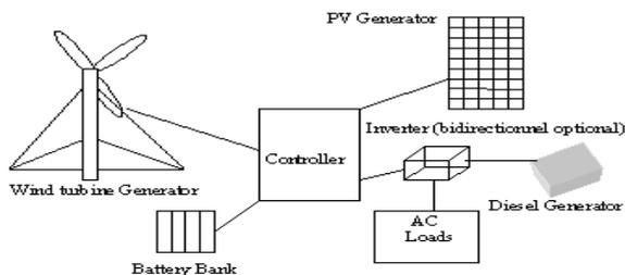
Figure 1: Schematic diagram of hybrid energy system.
