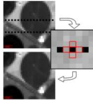
Fig 2: Modified horizontal noise algorithm in CHRIS sensor images
