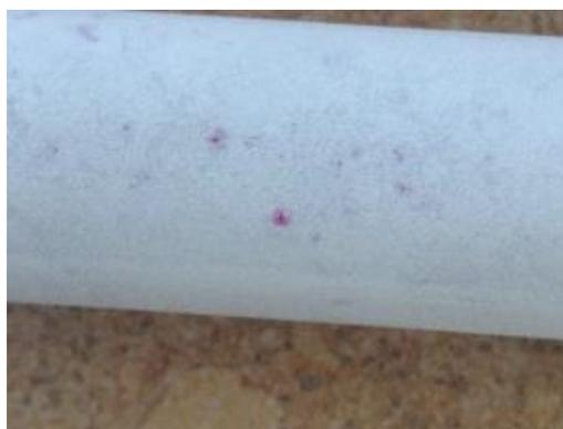
Fig. 3. Revelation of corrosion pitting through sweating-penetrant testing.
