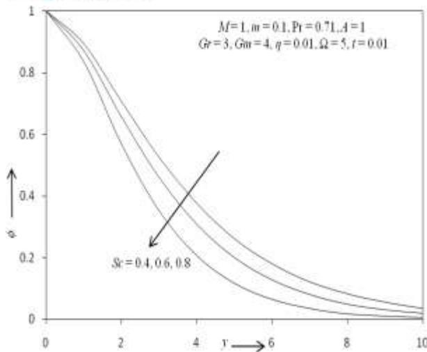
Fig - 19: The Concentration Profile for different Value of  $Sc$ .
