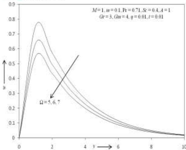
Fig. 13: The secondary velocity profile for different values of  $\Omega$ .
