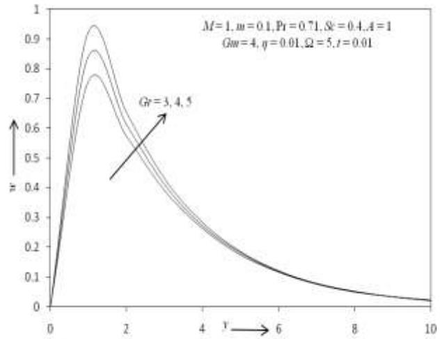
Fig - 11: The secondary velocity profile for different values of  $Gr$ .
