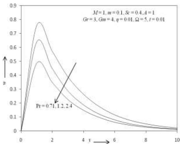
Fig. 15: The secondary velocity profile for different values of  $Pr$ .
