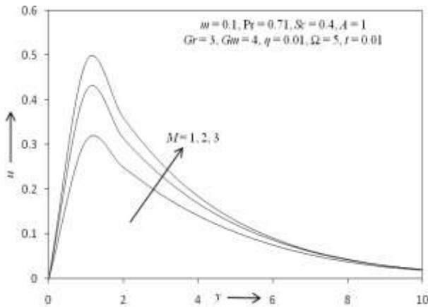
Fig - 1: The primary velocity profile for different value of  $M$ .
