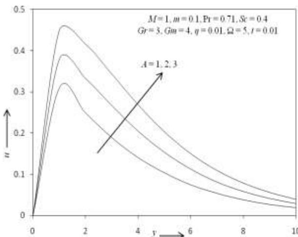
Fig - 8: The primary velocity profile for different value of  $A$ .
