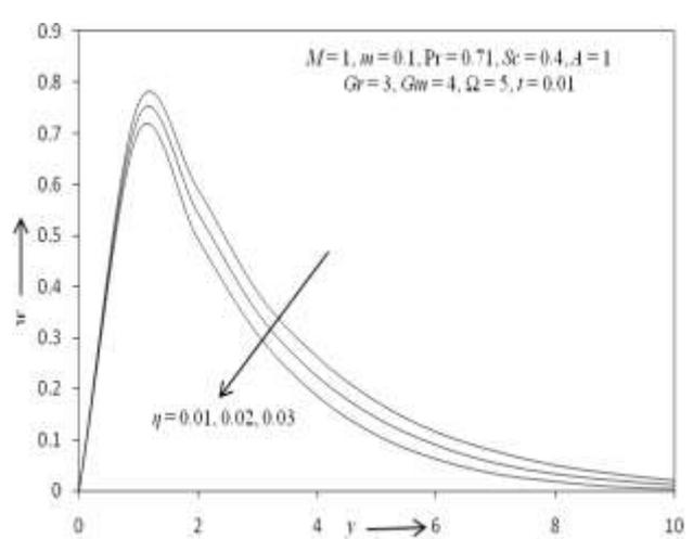
Fig. 18: The secondary velocity profile for different values of  $\eta$ .
