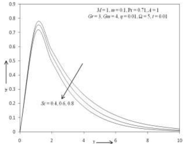
Fig. 16: The secondary velocity profile for different values of  $Sc$ .
