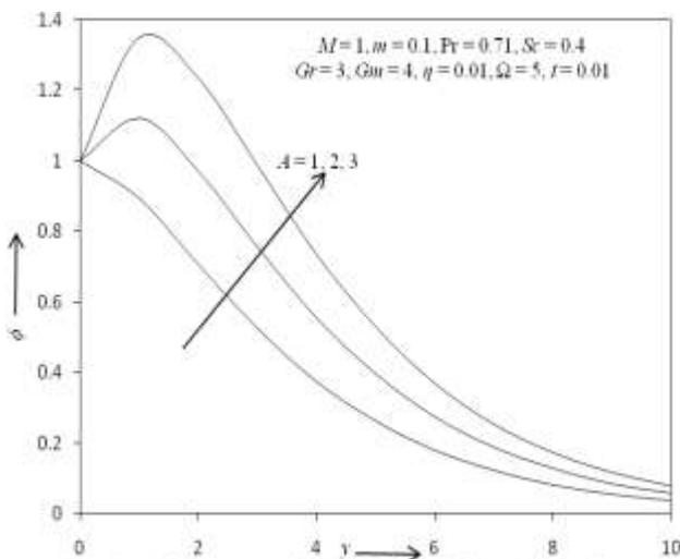
Fig - 20: The Concentration Profile for different Value of  $A$ .
