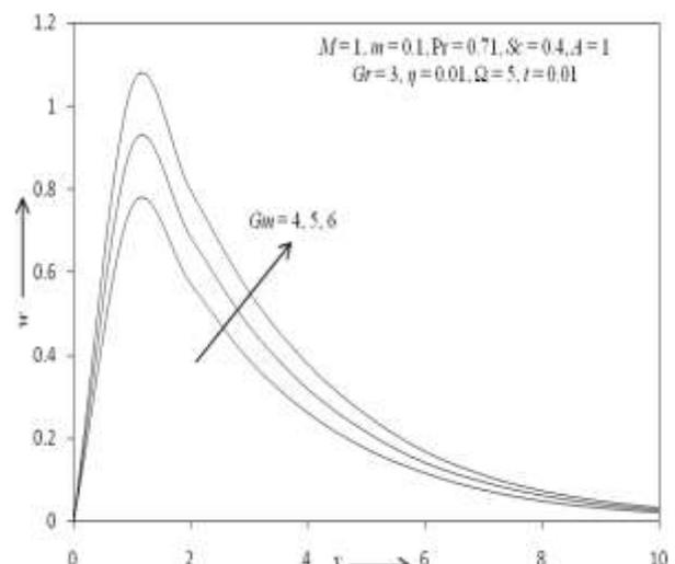
Fig - 12: The secondary velocity profile for different values of  $Gm$ .
