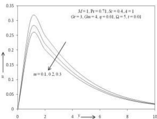
Fig - 3: The primary velocity profile for different value of  $m$ .
