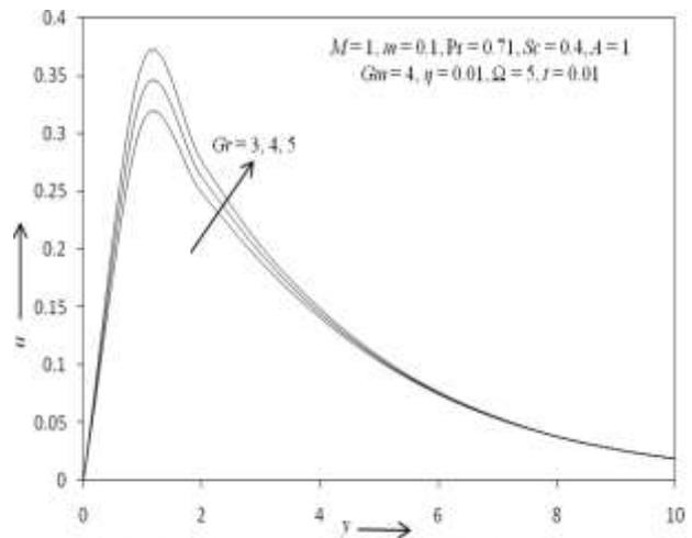
Fig - 5: The primary velocity profile for different value of  $Gr$ .
