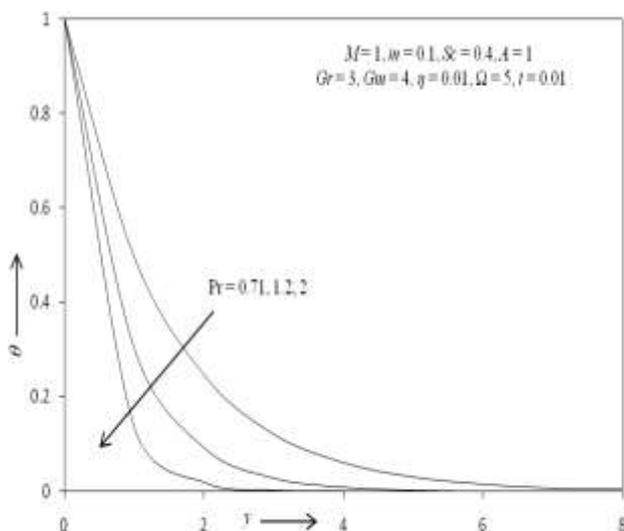
Fig - 21: The temperature Profile for different Value of  $Pr$ .
