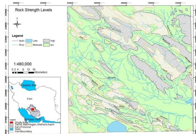
Fig.10. It shows HI value on rock strength map. There are HI anomalies in some basins such as basin 4, 3, 8, 28, 26 and 27.
