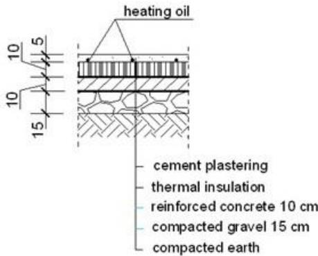
Fig. 1. Structure of floor covering.
