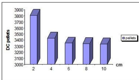
Fig. 3. Amount of DC for various thickness of thermal insulation in pellets as fuel.
