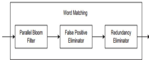
Fig.2. Tuesday substages of FPGA-based accelerator for the matching word BLASTN [7]
