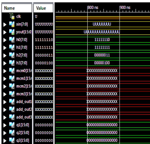
Fig. 8 . FIR bandpass filter waveforms
