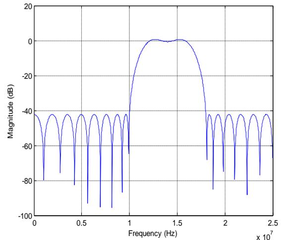
Fig. 3 . FIR bandpass filter
