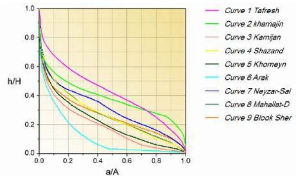
Fig.5. Hypsometric curves of nine basins, (A) is the total surface area within the basin above a given line of elevation (h), and (H) is the highest elevation of basin.
