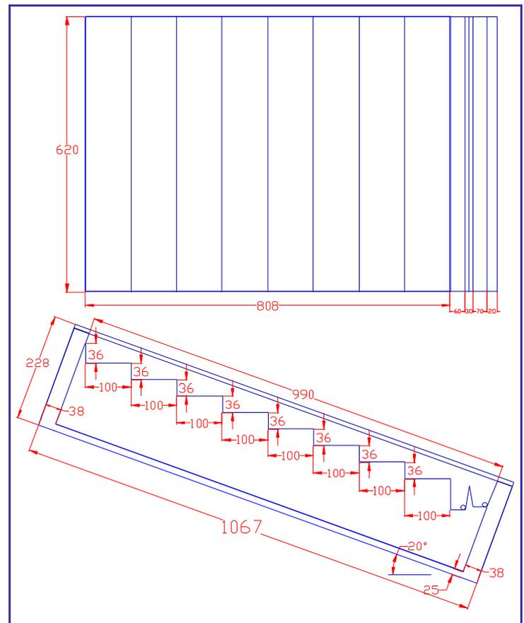
Fig.2: Schematic diagram of the stepped type solar still
