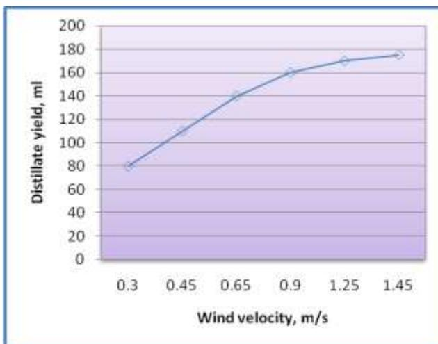
Fig. 7: Variation of distillate yield with wind velocity for solar still H with fins provided over the basin
