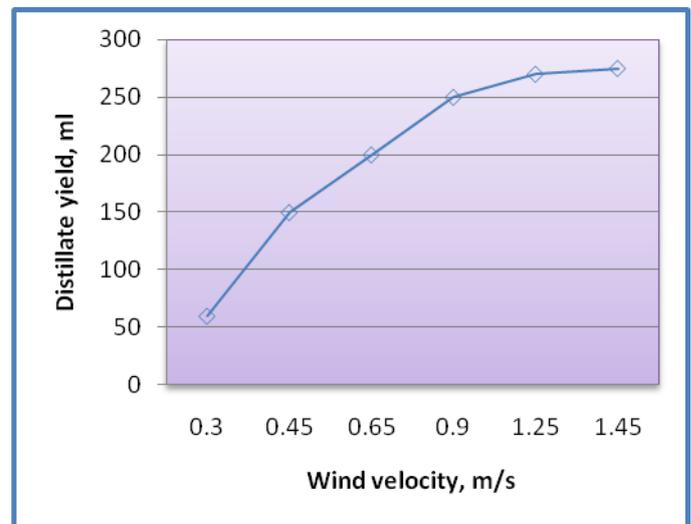
Fig. 4: Variation of distillate yield with wind velocity for solar still A with 5 mm depth of water
