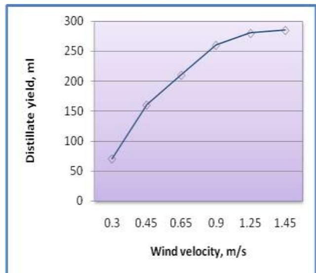
Fig. 5: Variation of distillate yield with wind velocity for solar still D with 3.5 mm glass cover thickness
