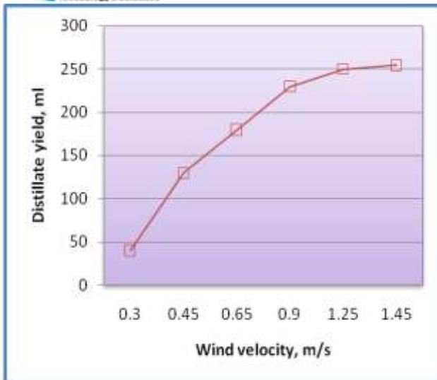
Fig. 6: Variation of distillate yield with wind velocity for solar still E with concave basin surface
