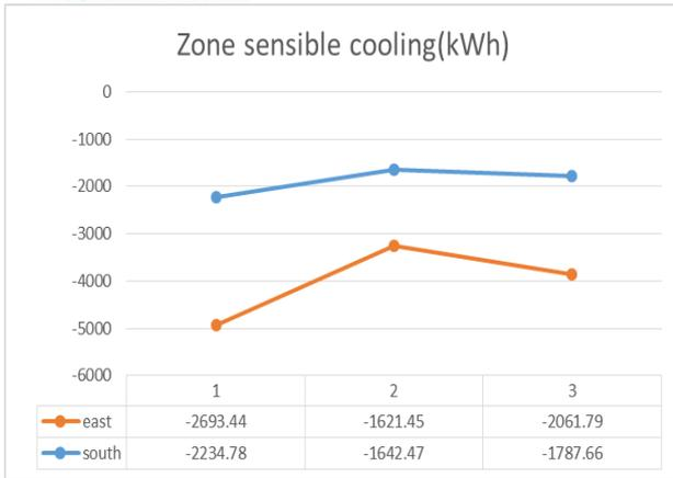
Fig.5. Evaluation of overhang in windows facing the South and East with WWR=40%
