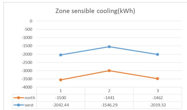
Fig.7. Evaluation of the overhang on windows facing the North and West in cold six-month of year with WWR=20%
