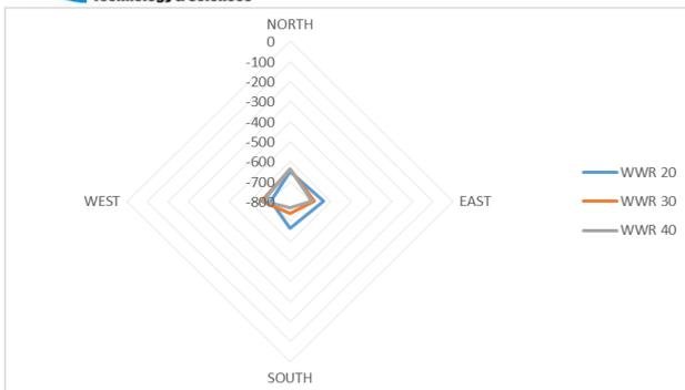
Fig.2. The rate of energy dissipation (kWh) in the cold six-month of year
