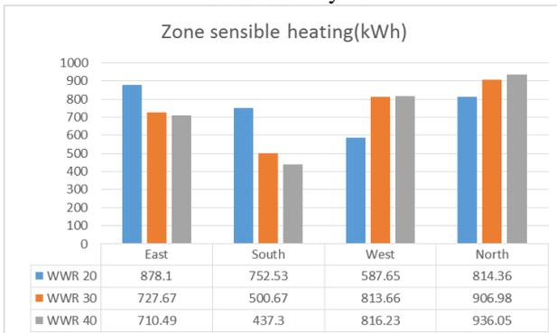
Fig.3. Zone sensible heating (kWh) in cold six-month of year in different geographical directions
