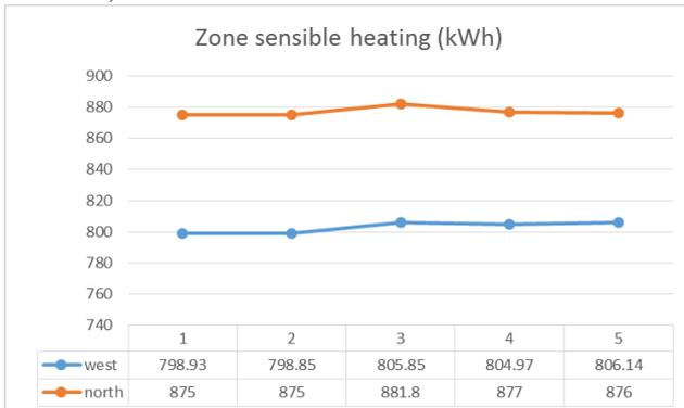
Fig.6. Analysis of the proportions of window facing the North and West in cold six-month of year with WWR=20%<sup>3</sup>
