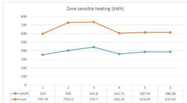
Fig.4. Zone sensible heating (kWh) in cold six-month of year in windows facing the South and East with WWR=40%<sup>2</sup>
