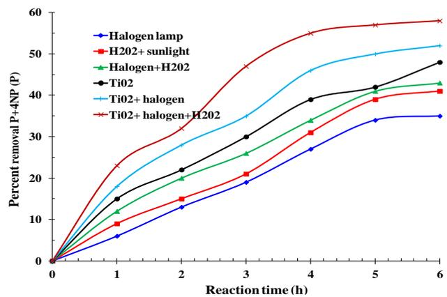
Figure 4. Effect of different process on percent removal of P in binary mixture at C<sub>0</sub>= 100 mg/l; pH=11; for 4h as reaction time.
