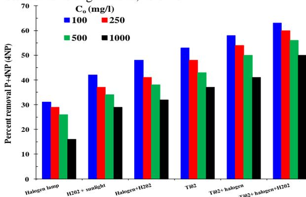
Figure 1. Effect of various initial concentration on percent removal of 4NP in the binary mixture at pH=11; 4h as reaction time.
