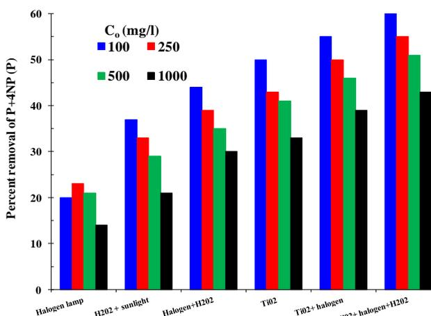
Figure 2. Effect of various initial concentration on percent removal of P in the binary mixture at pH=11; 4h as reaction time.
