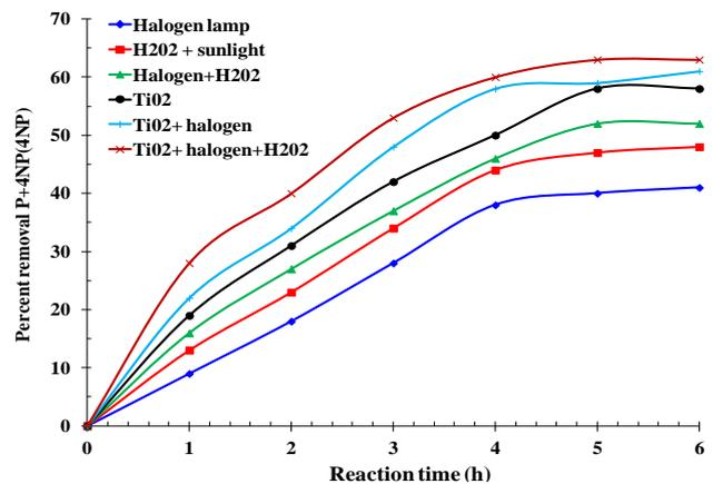
Figure 3. Effect of different process on percent removal of 4NP in binary mixture at C<sub>0</sub>= 100 mg/l; pH=11; for 4h as reaction time.
