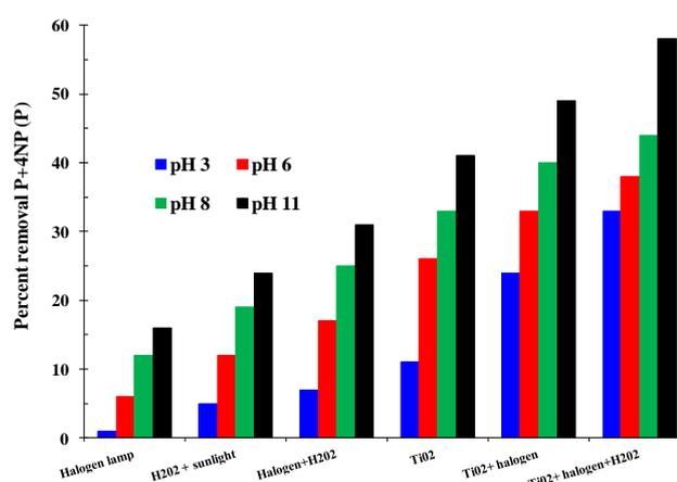
Figure 6. Effect of different pH on percent removal of P in binary mixture (P+4NP) at  $C_0=100$  mg/l; 4h reaction time.
