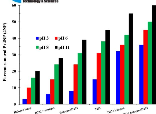
Figure 5. Effect of different pH on percent removal of 4NP in binary mixture (P+4NP) at  $C_0=100$  mg/l; 4h reaction time.
